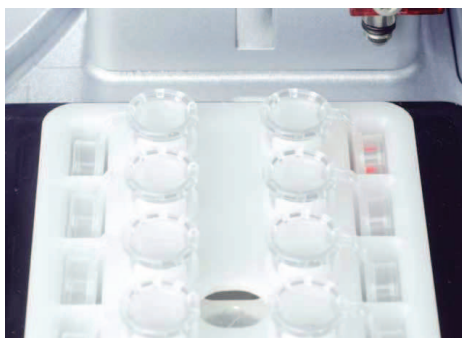
Figure 2. Hands-free sample lysis. The integrated shaker enables fully automated lysis of up to 12 samples.
