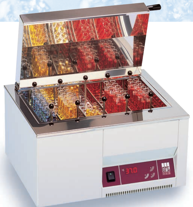
1013 Water Bath with circulation system, 14 litres
