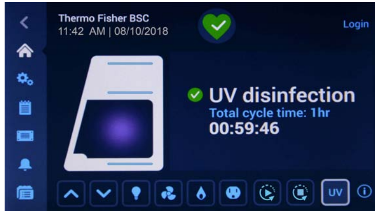
Figure 46 Main Screen: “UV disinfection” running
