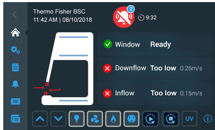
Figure 60 Main Screen after two Cycles of Alarm Ticker Message
