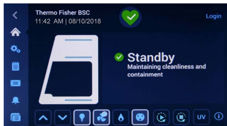
Figure 36 Main Screen - Unit in Standby
