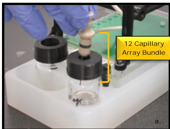
Figure 8-71a and b. Fragment Analyzer Wet Station™ 12-Capillary Array Bundle in Storage Bottle
