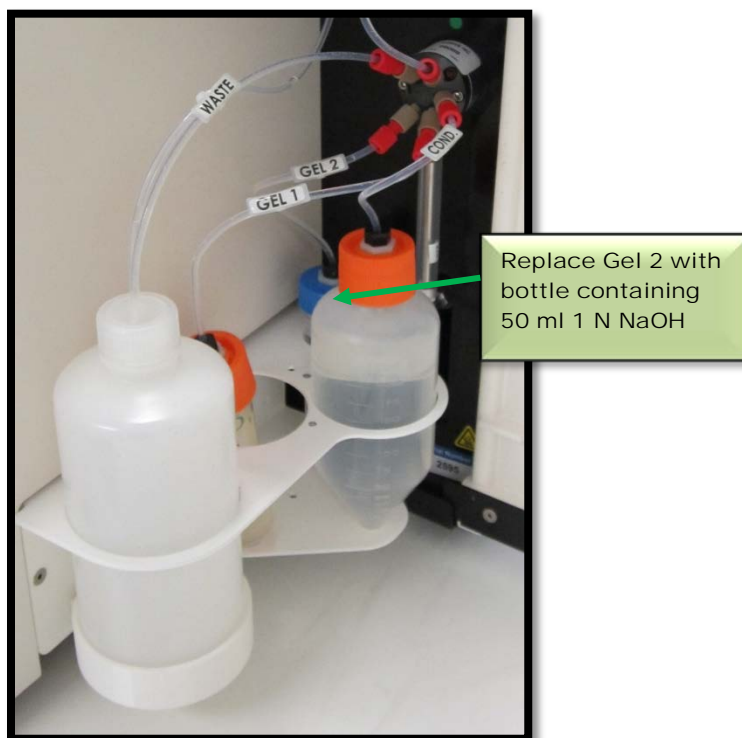
Figure 9-22: Instrument Side Compartment. Replace Gel 2 with 1 N NaOH Solution
